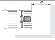
RECOMMENDED - A space of not less than one fan diameter [D] should be allowed at the inlet.
