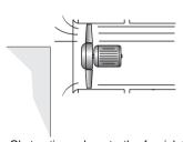
WRONG - Obstructions close to the fan inlet also starve the impeller of air.
