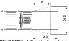
RECOMMENDED - A 2D duct length or a discharge evase of dimensions illustrated reduces system discharge losses.
