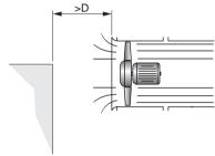
RECOMMENDED - A space of not less than one fan diameter [D] should be allowed at the inlet.
